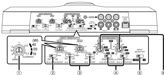
This is a 4 channel amplifier including 2 stereo amplifiers in a body. One amplifier is referred to as amplifier A and the other is amplifier B. This unit is compatible with a large variety of systems by combining the switches and functions described in the following.
